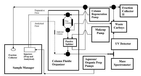
Figure 1. Configuration of Waters autopurification system.
